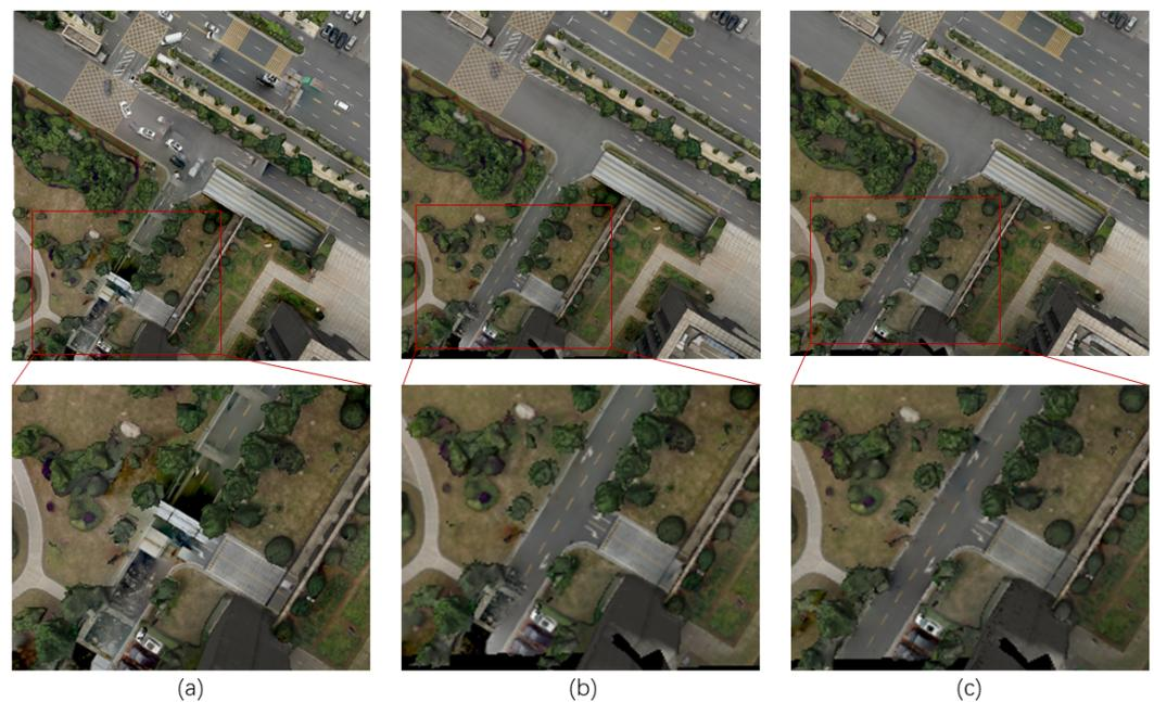
**Figure 7.** Results comparison without occlusion detection model. (a) results of experiments without image consistency detection; (b) results of the method of mvs-texturing; and (c) results of our method.
