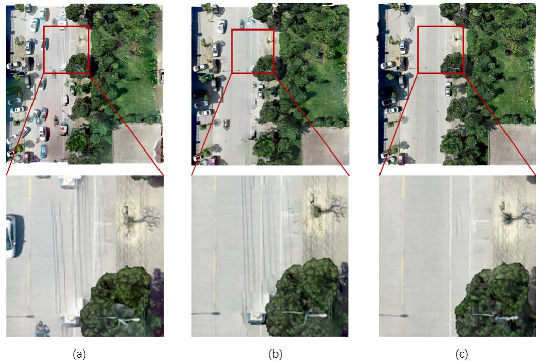
**Figure 6.** Comparison of texture-mapping results of the road wires of in dataset TJH-0078. (a) results of experiments without image consistency detection; (b) results of the method of *mvs-texturing*; and (c) results of our method.
