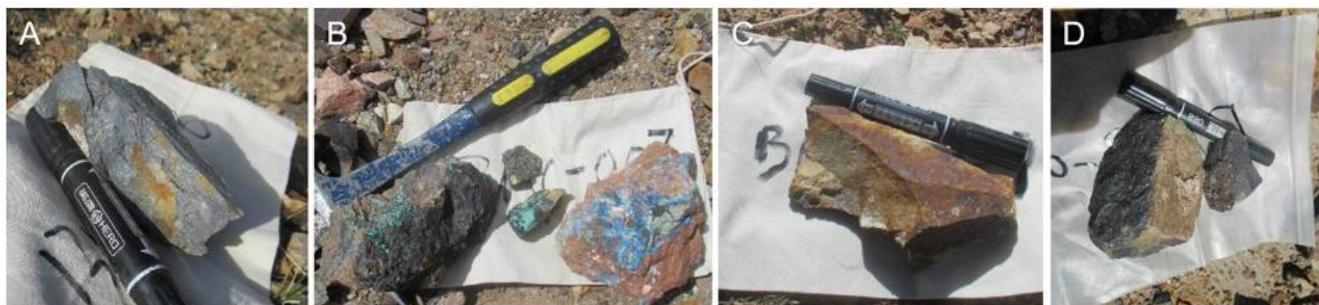
Figure 17. Field photographs of the study areas: (A) chalcopyrite-bearing diorite in Tiegelong; (B) malachite (left and middle) and azurite (right) in Duobuza; (C) Gossan in Gaerqin; and (D) chalcopyrite mineralization in Naton.
