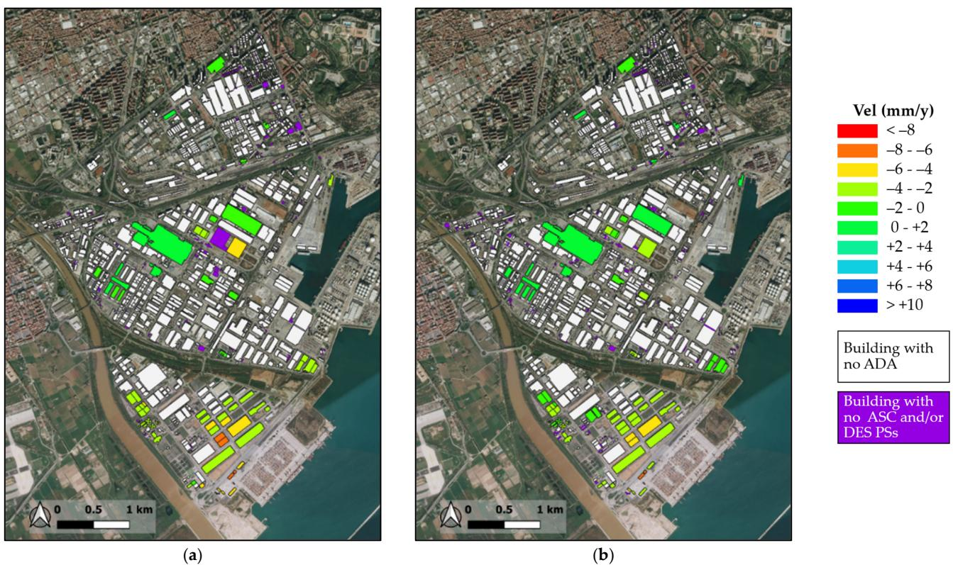
**Figure 7.** Maps of buildings in *Zona Franca* area with an average value of mean deformation velocity along (a) ascending and (b) descending orbit. The violet polygons represent buildings with lack of PSs.
