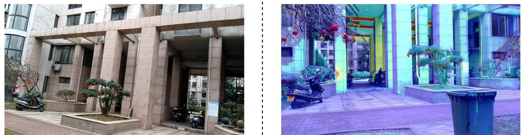
**Figure A3.** The left image illustrates the scene used for LiDAR-camera calibration. The right image shows the result of projecting the LiDAR point cloud onto the image using extrinsics between LiDAR and camera.
