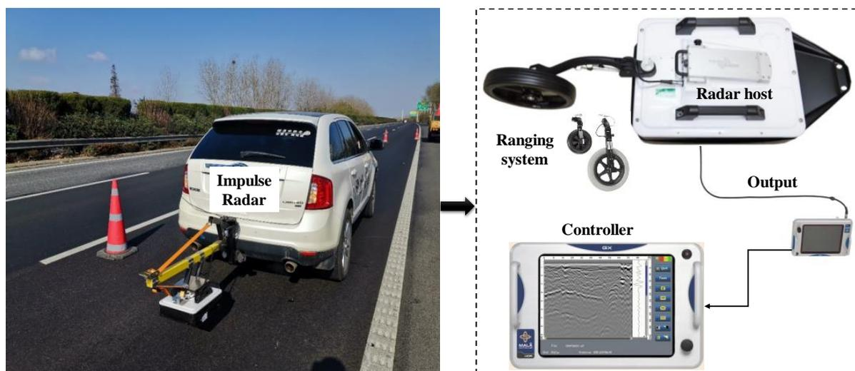
**Figure 3.** GPR detection for pavement structure conditions.
