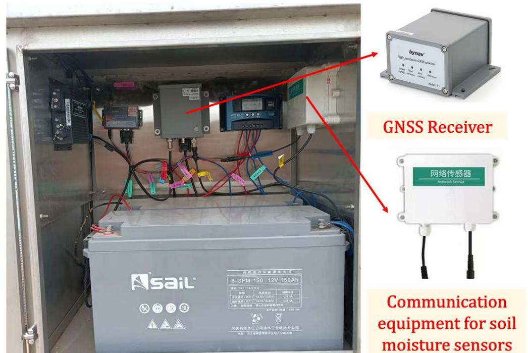
**Figure 8.** GNSS receiver diagram and Soil moisture sensors communication equipment.
