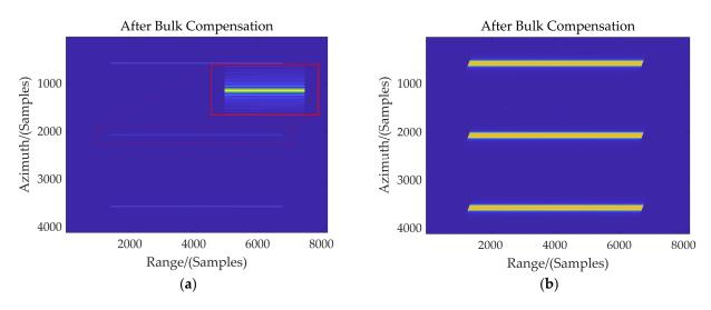
**Figure 3.** (**a**,**b**) Raw echo signals in two-dimensional time domain after bulk compensation for central and non-central range cells, respectively.
