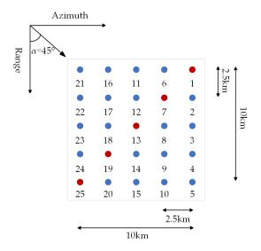
Figure 7. Point matrix on-the-ground scene used in the simulation.
