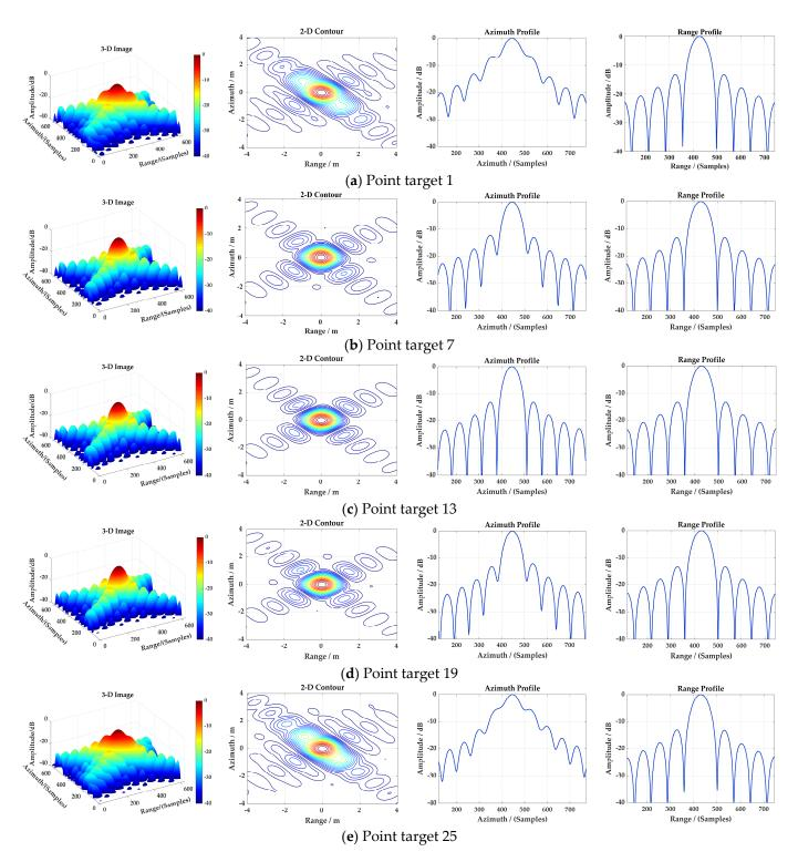
**Figure 10.** (**a**–**e**) The imaging result of the chosen point targets 1, 7, 13, 19 and 25 using the LRWC-based algorithm, respectively.
