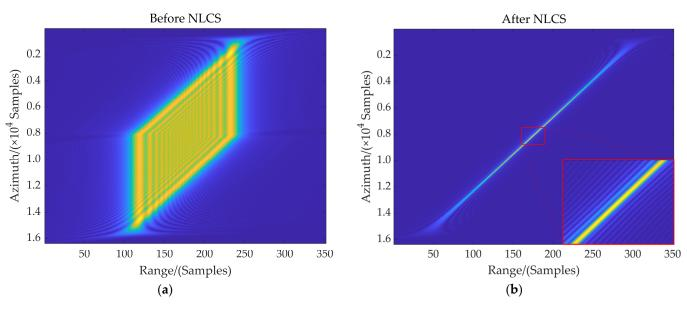
**Figure 4.** (**a**,**b**) Range compression results for the range marginal target in RD domain before and after NLCS, respectively.
