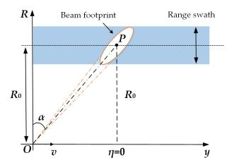
Figure 1. Geometry model of the high-squint airborne SAR system.
