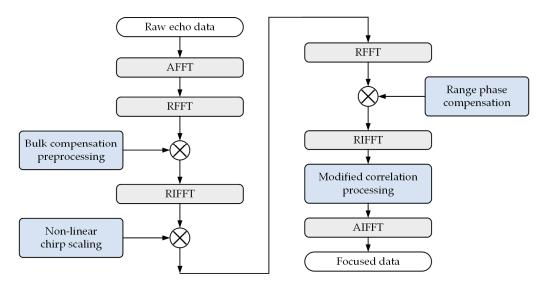
Doppler phase modulation compensation and the range-variant cubic phase modulation compensation, and the focused SAR data can be acquired at the end via an AIFFT operation.
