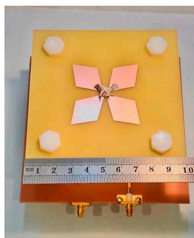
**Figure 7.** The E5a/b NJBW antenna verification prototype.
