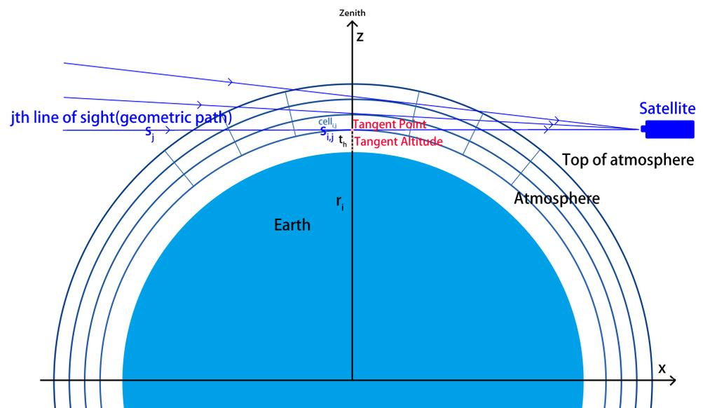
**Figure 4.** Limb observation schematic.
