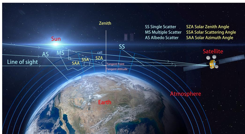
**Figure 1.** Limb observation geometry. AS, albedo scatter; MS, multiple scatter; SS, single scatter; SAA, solar azimuth angle; SSA, single scattering angle; SZA, solar zenith angle.
