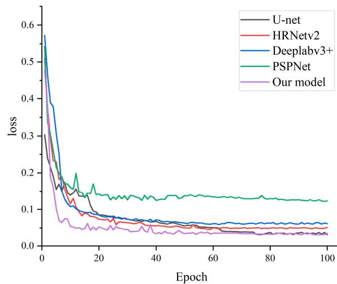
**Figure 8.** Curves of loss values of different models as the number of iterations increases in the training process on the WHU dataset.
