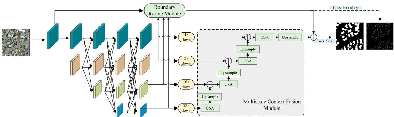
**Figure 1.** The structure of multi-scale boundary-refined HRNet (MBR-HRNet). The MBR-HRNet consists of two main components: the boundary-refinement module (BRM) and multi-scale context fusion module (MCFM). The CSA module represents channel-spatial attention.
