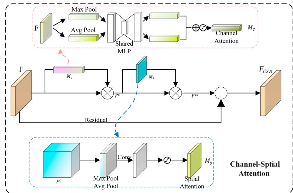
Figure 5. Structure of channel-spatial attention (CSA).  $F$  represents the input, while  $F_{CSA}$  represents the feature map obtained after passing through the CSA layer.
