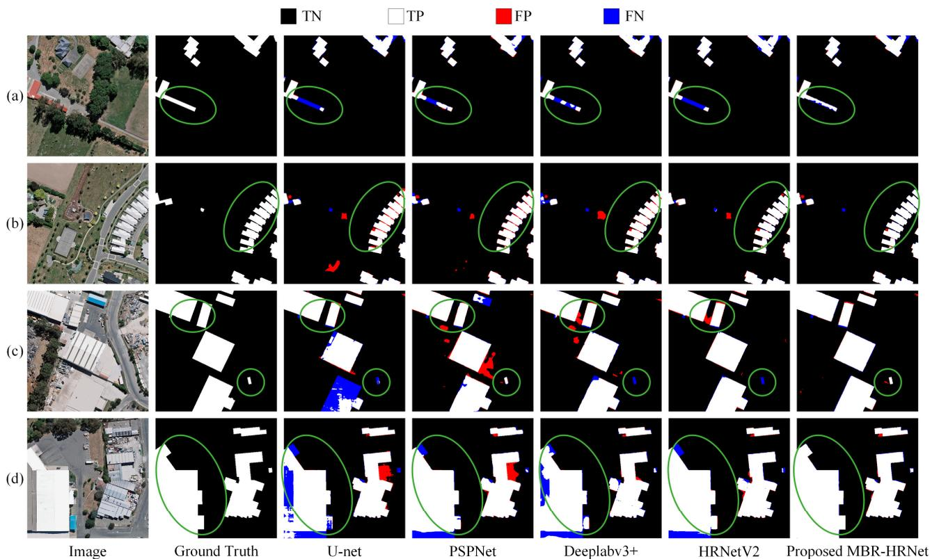
**Figure 10.** (a–d) The building extraction results of the proposed model on the WHU dataset. TN indicates the background, TP indicates the accurately detected building area, FP indicates the wrongly detected building area, and FN represents the parts of the building that were missed.
