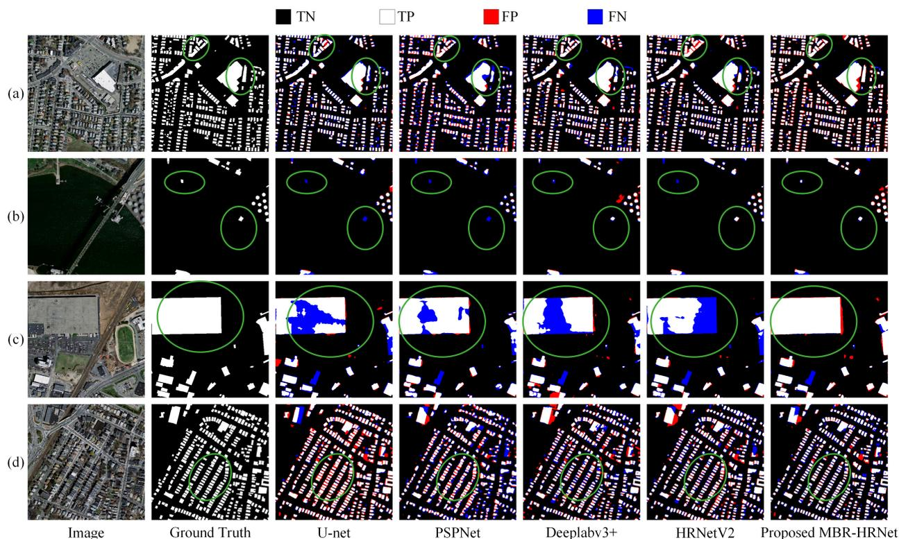
**Figure 11.** (a–d) The building extraction results of the proposed model on the Massachusetts dataset.
