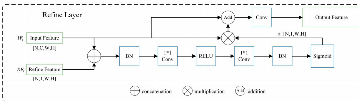
Figure 3. Structure diagram of the refine layer in the BRM.
