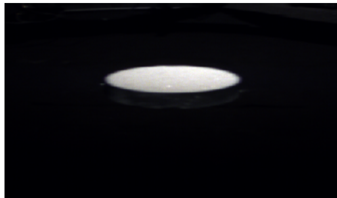
Figure 5. Example hyperspectral Raw DN output image for a 500–600 \mu\text{m} Nepheline sample with polarizer zenith angle of 0 deg and illumination zenith angle of 50 deg. Displayed RGB bands selected from the hyperspectral imagery are, respectively, band 156 (650.99 nm), band 94 (550.231 nm), and band 33 (451.097 nm).
