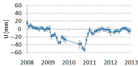
**Figure 7.** Change in the vertical component of the SLR station Wettzell (Germany) due to station bias.
