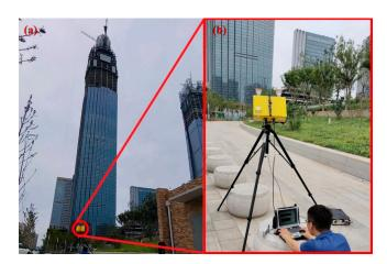
**Figure 4.** Deformation monitoring diagram of Main Tower. (a) Ground view of Main Tower from the location of the IBIS system; (b) View of the IBIS-S system on S2.
