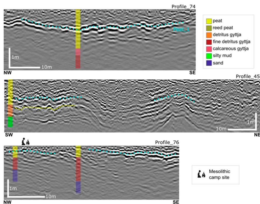
**Figure 4.** GPR profiles belonging to the survey performed at Duvensee (200 MHz) in comparison with the stratigraphy. The internal layering of the peat is depicted by a cyan dotted line. For the profile location, see Figure 1b. The colored bars represent stratigraphic information from corings.
