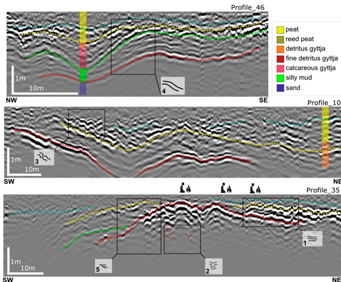
**Figure 8.** GPR profiles showing the different GPR facies classified in Figure 7. The different symbols are re-reported for comparison and the different sediments as well. The dashed lines indicate the different sediment interfaces reported in [6,16] and in Figure 3 of this study. The illustrated profiles are from the 200 MHz survey.
