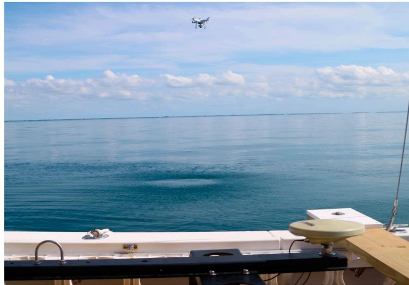
**Figure 5.** UAS image acquisition over Florida Keys project site with Phantom 4 Pro. In the foreground is the starboard gunwale of the Mote Marine Laboratory dive boat from which takeoff and landing were performed.
