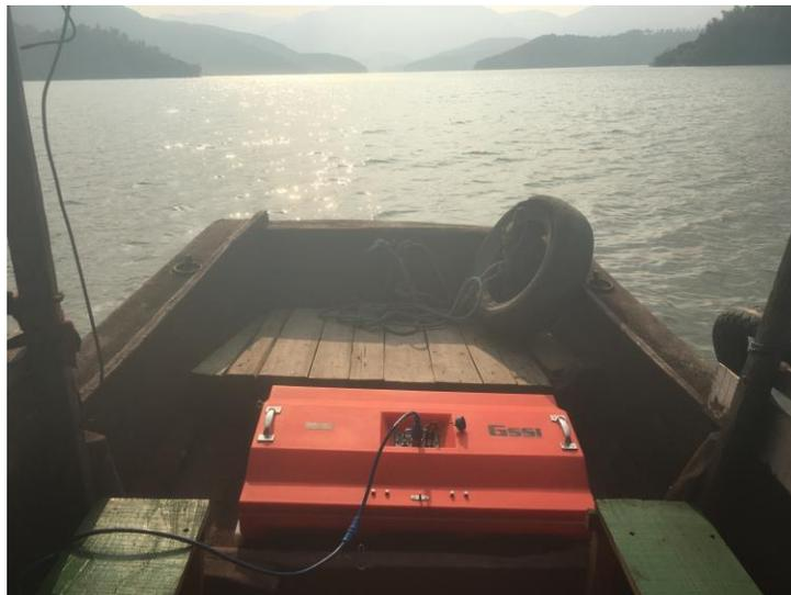
**Figure 5.** An on-site photo using GSSI SIR-4000 GPR.
