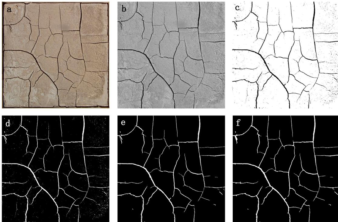
**Figure 4.** Standardized preprocessing process for crack images. (a) Crack image after geometric correction, (b) grayscale crack image, (c) binarized crack image, (d) inversed binary image, (e) denoised crack image, (f) crack image after bridging process.
