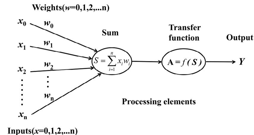
Figure 6. A simple schematic diagram of artificial neural network.
