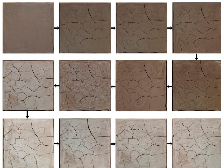
**Figure 3.** Cracking process of a typical soil sample in this study.
