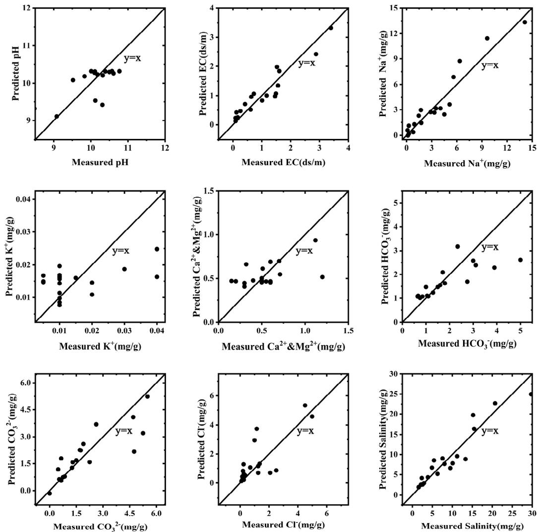
Figure 9. Fitting results of measured and predicted values using BP neural network method.
