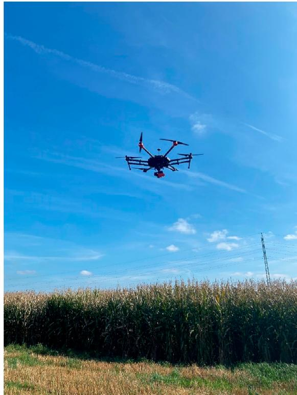
**Figure 3.** Capturing the image data with a drone-mounted RedEdge camera.
