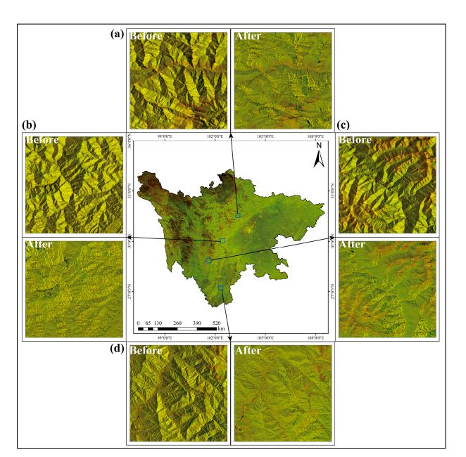
**Figure 4.** The comparison of topographic corrections for Sentinel 1B. (**a**). Before and after topographic corrections in region (**a**). (**b**). Before and after topographic corrections in region (**b**). (**c**). Before and after topographic corrections in region (**b**). (**c**). Before and after topographic corrections in region (**d**).
