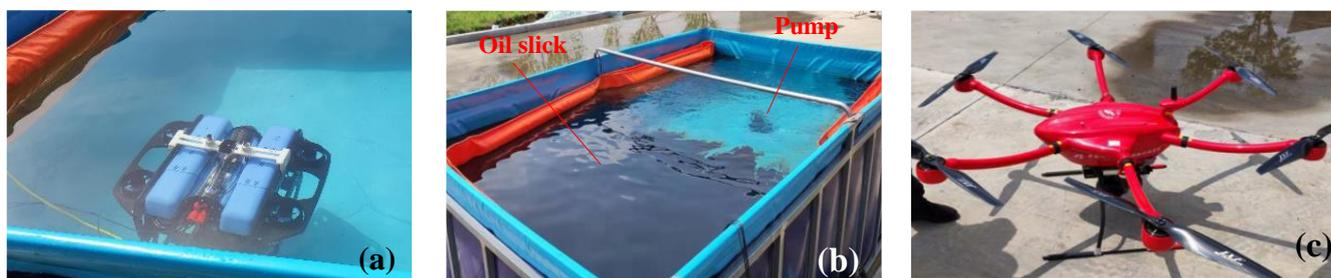
**Figure 5.** (a) The ROV carrying two 5 MHz ultrasonic transducers dived in the tank before adding oil, (b) the oil slick boomed in the water tank, (c) the six-rotor drone platform with an optical camera used for capturing images.
