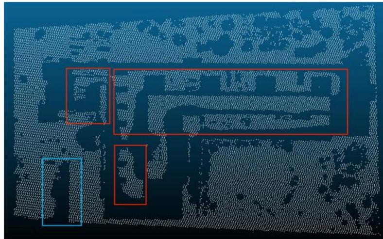
**Figure 22.** Cloth Simulation Filter (the red box selection area indicates that the non-ground point is used as the ground point retention area; the blue box selection area indicates that the ground point is used as the non-ground point removal area).
