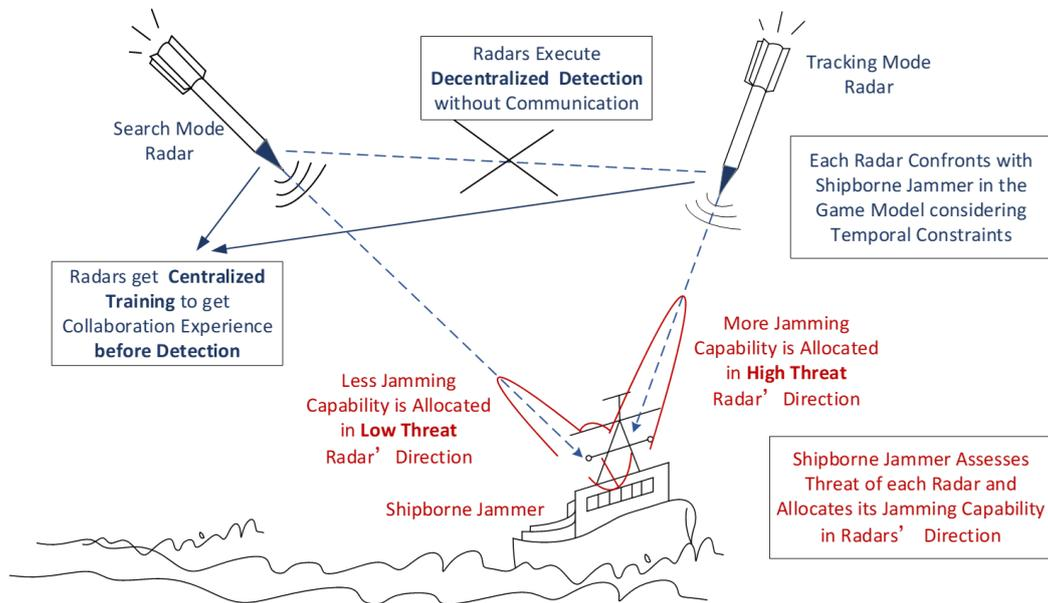
**Figure 1.** A schematic of the detection of a naval vessel by collaborative radars.
