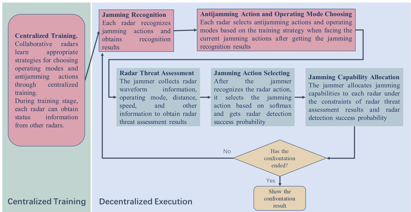
**Figure 2.** Flowchart of the MADDPG algorithm in multi-missile-borne radars vs. the shipborne jammer.
