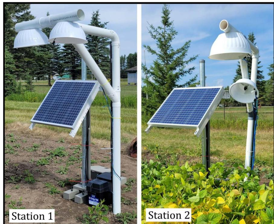
**Figure 2.** Camera Station Setups at different angles; cameras were operated using the power generated from a battery and a solar panel at each station. Raspberry Pi micro-computers were used to automate the image acquisition process.
