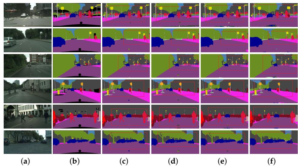
**Figure 4.** Comparison of the visual segmentation results of our proposed MPCNet with the other three methods for the Cityscapes dataset: (a) Image. (b) Ground Truth. (c) PSPNet [31]. (d) OCNNet [52]. (e) DeepLabv3+ [33]. (f) Ours.
