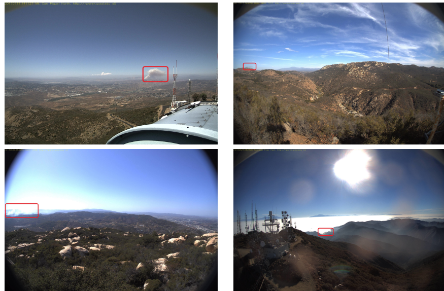
Figure 1. Sample images with smoke from the FIgLib dataset. The red bounding box indicates the location of the smoke plume. (Top left) Very apparent smoke plume; (top right) extremely faint smoke observed at a distance from the camera; (bottom Left) smoke blending into the area with strong glare; (bottom right) smoke with misleading haze.
