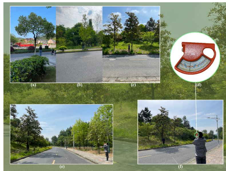
Figure 2. Traditional field survey. (a–c) CC, GB, and YD trees to be measured. (d) Blume–Leiss gauge. (e,f) Measuring the tree heights using the Blume–Leiss gauge.
