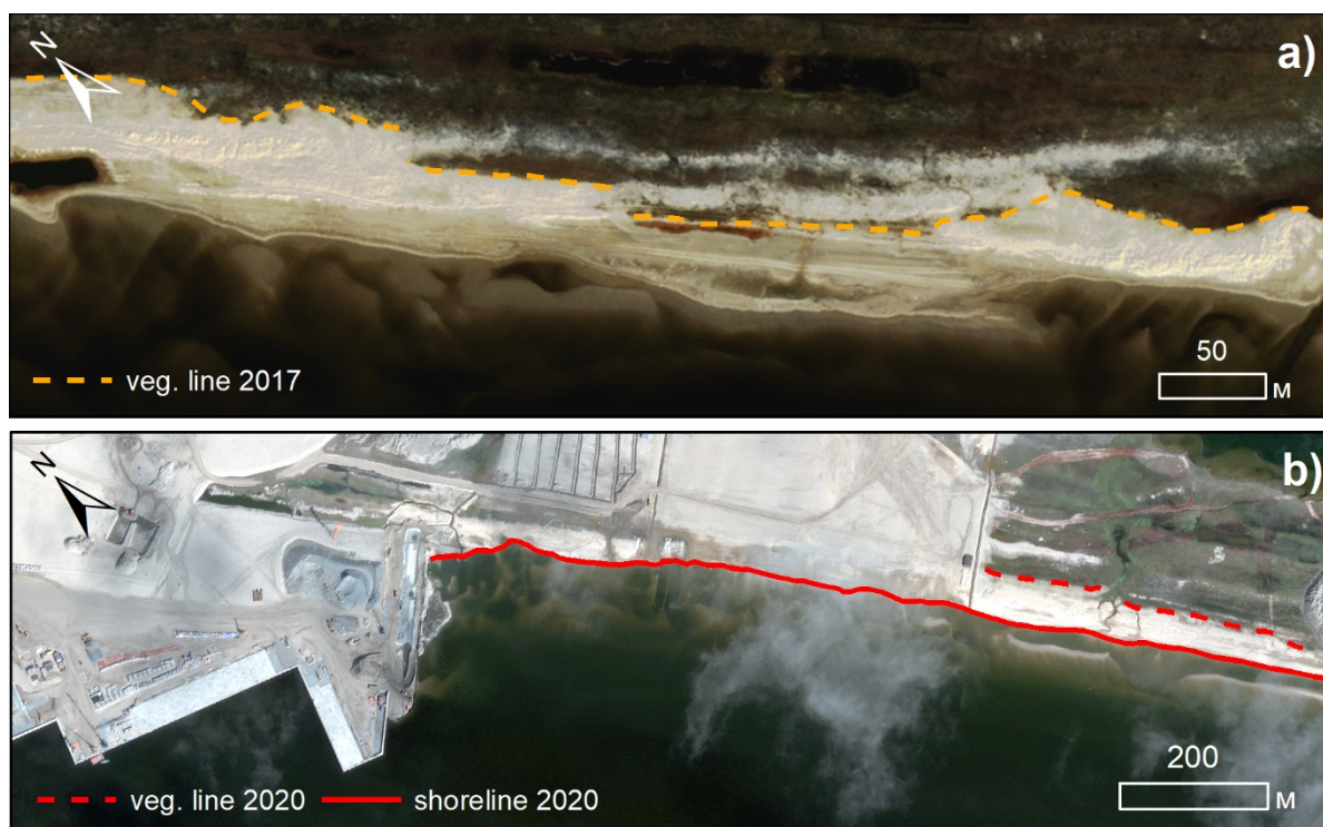
Figure 3. Challenging tracing of coastal lines position: (a) due to sandy aeolian cover on the laid surface (WV-2 2012); (b) due to construction in the coastal zone (WV-2 2020).
