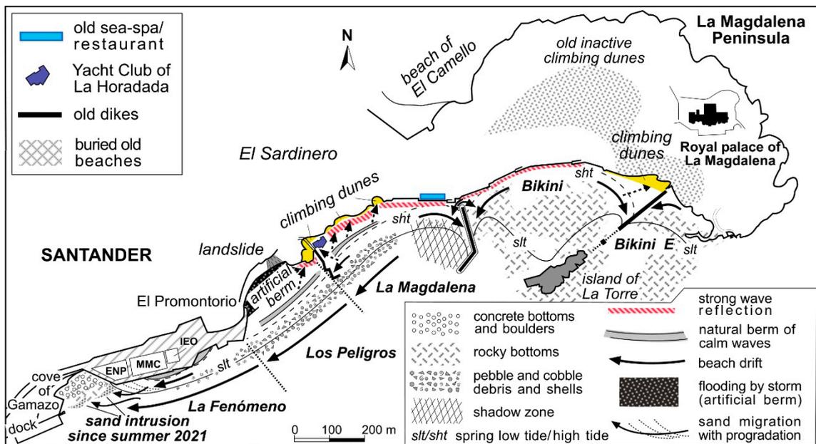
**Figure 10.** Morphodynamic conceptual model after the construction of the breakwater (2018), highlighting the following main processes: reflection in the upper beach during storm, which has only been artificially recovered; westward beach drift; and aeolian transport to the small outcrops of climbing dunes mainly of Los Peligros and La Magdalena. The former cove of Gamazo, with calcareous and concrete bottoms and boulders, is turning into a sandy beach.
