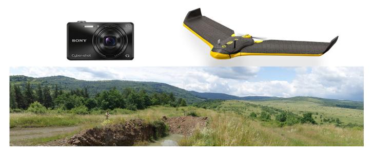
**Figure 2.** A broader view of the study area (**bottom**); the senseFly eBee equipped with a consumergrade DSC-WX220 digital compact camera (**top**).
