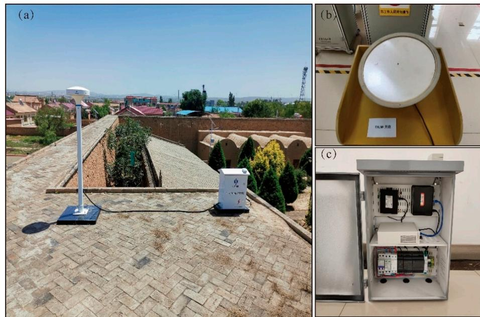
**Figure 2.** The field scene at site TJZ (a); that is equipped with a fast antenna (b); and controlling box (c).
