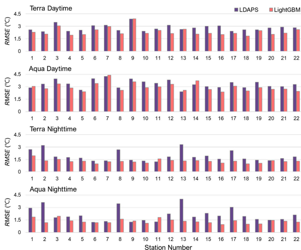
Figure 6. RMSEs for cloudy-sky LSTs from the LDAPS and proposed LightGBM models against the bias-corrected in situ LST measurements for each ASOS. Please refer to Figure 1 for station numbers.
