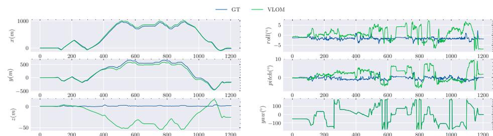
**Figure 14.** Changes in the position and orientation contrasted with the ground truth on the RS dataset.
