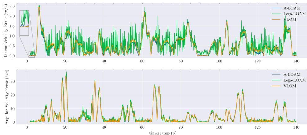
**Figure 15.** Comparison of velocity errors on the OS dataset, including the linear velocity error (**top**) and angular velocity error (**bottom**).
