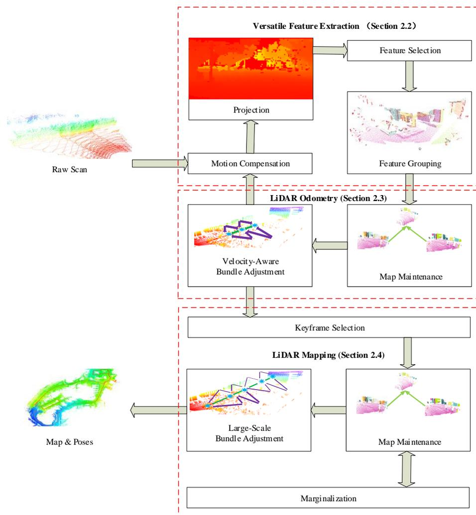
**Figure 2.** Overview of our SLAM system, which has three main parts: a versatile feature extraction module, a LiDAR odometry module, and a LiDAR mapping module.
