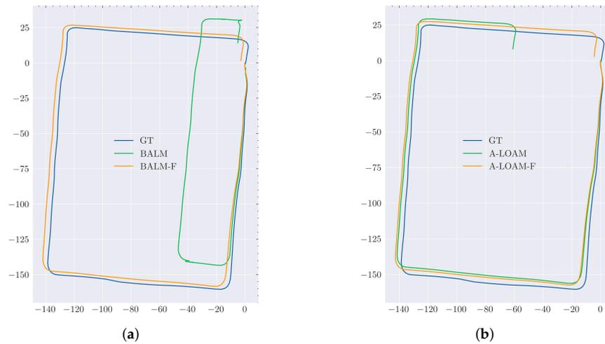
**Figure 9.** There are clearly large errors in the origins of BALM (a) and A-LOAM (b). By replacing the feature extraction module with our scheme, the new algorithms, BALM-F (a) and A-LOAM-F (b), achieve impressive performance improvements.
