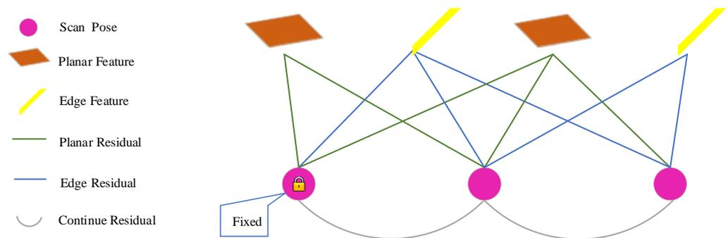
**Figure 5.** Illustration of our graph for odometry optimization. The first pose serves as a prior and is fixed during the optimization process. The planar and edge features impose constraints on all scans that observe them, while the constant motion model imposes constraints on neighboring scans.
