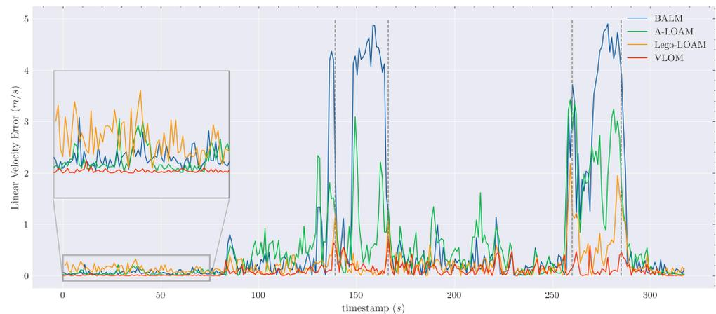
**Figure 10.** Comparison of the linear velocity errors on *HK-Data20190117*. VLOM has a very low error throughout the sequence, especially during the initial phase shown in the magnified area. Lego-LOAM is more accurate than the other methods; however, it has a poor performance in the areas marked by the gray dotted line.
