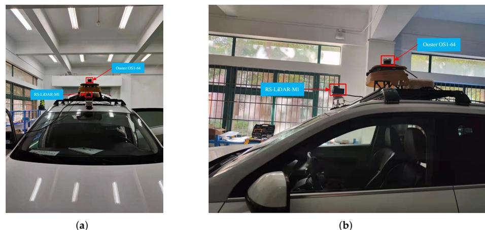
**Figure 12.** Experimental platform. (a) Front view. (b) Side view. Ouster OS1-64 and RS-LiDAR-M1 were placed on the roof and front of the vehicle, respectively.
