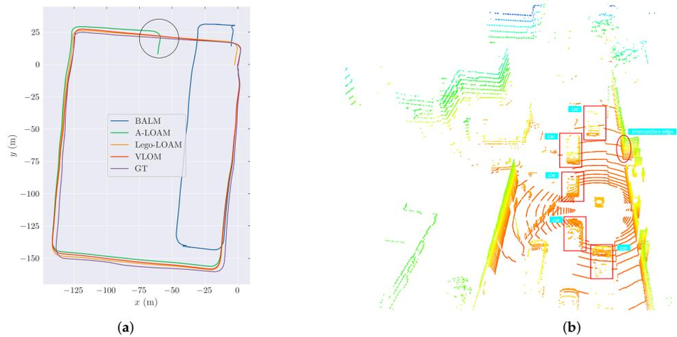
**Figure 8.** (a) compares the estimated trajectories with the ground-truth trajectories in the HK-Data20190117 dataset. Note that all trajectories were aligned to the ground truth according to the EVO library. (b) shows a point cloud acquired at the position where A-LOAM begins to fail, which is marked by the circle in (a).
