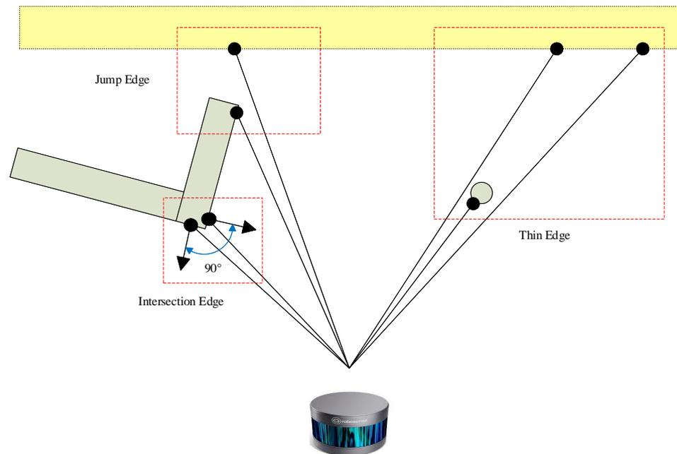
**Figure 3.** Our edge feature selection scheme. An intersection edge is a planar point with a smaller depth than its neighboring points and a larger angle, e.g.,  $90^\circ$ , between the corresponding normal vectors. A jump edge is a plane point with a much smaller depth than its neighboring points. A thin edge is a point with two neighbors in the same row or column that have much larger depths. The depth is infinite if the yellow plane with the dashed boundary does not exist.
