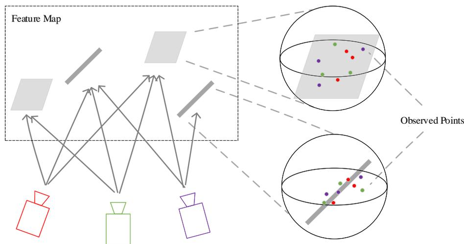
**Figure 4.** A map in 3D space. The two spheres on the right show the details of the planar and edge features. The different colored points in the spheres correspond to the LiDAR scans of the same color.
