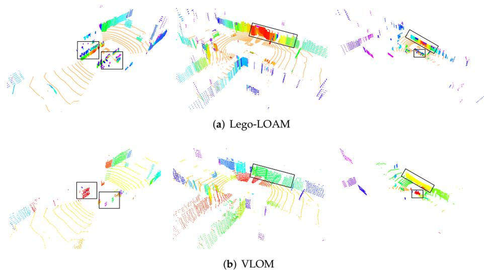
**Figure 7.** Segmentation results of Lego-LOAM (a) and VLOM (b). The various colors represent different planes. The rectangle in the image indicates some differences between Lego-LOAM and VLOM. The continuous color in Lego-LOAM indicates that each plane is divided into several parts.
