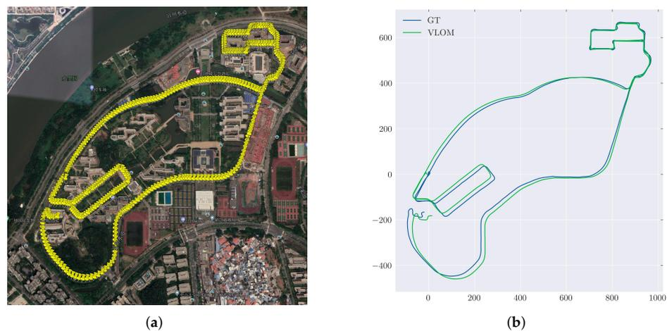
**Figure 13.** Trajectory of the dataset acquired with RS-LiDAR-M1. (a) Ground truth aligned to Google Earth from a top view. (b) Comparison of the VLOM trajectory and the ground truth. The results are presented in meters.
