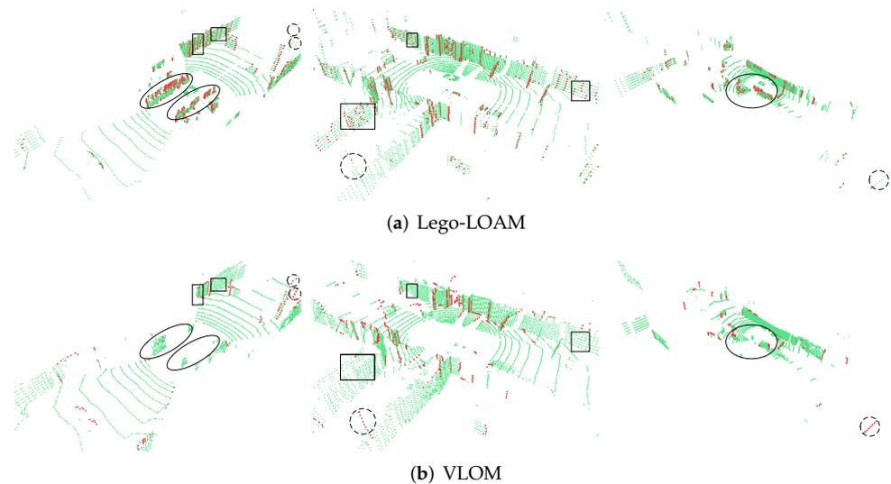
**Figure 6.** Comparison of the feature extraction results with Lego-LOAM and VL0M. (a) Features extracted with Lego-LOAM and (b) features extracted with VL0M. The green dots indicate planar feature points, while the red dots indicate the edge feature points. We marked some regions at the corresponding positions to compare the details of the two results.
