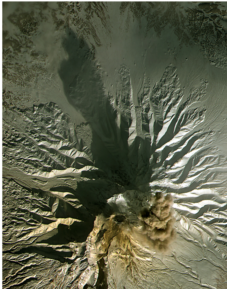
Figure 11. Detail of an scene by the Advanced Spaceborne Thermal Emission and Reflection Radiometer (ASTER) acquired on 17 February 2008. We applied the the shadow-height methodology to calculate the height and vertical velocity of an ash plume at Shiveluch Volcano in Kamchatka, Russia.
