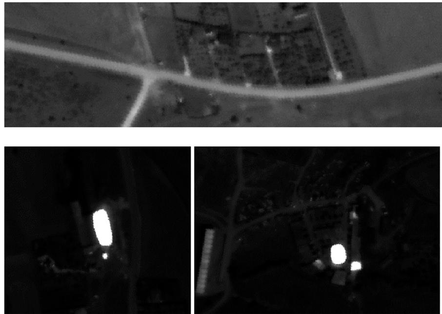
**Figure 13.** Examples of edge jitter (**above**) and saturation (**below**) artefacts in SkySat data.
