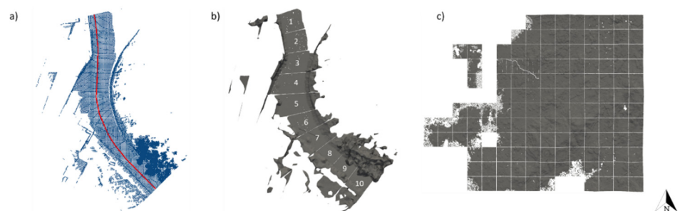
Figure 14. EP9703 road: (a) point cloud with vehicle trajectory, (b) MLS triangle mesh segments, and (c) ALS triangle mesh.
