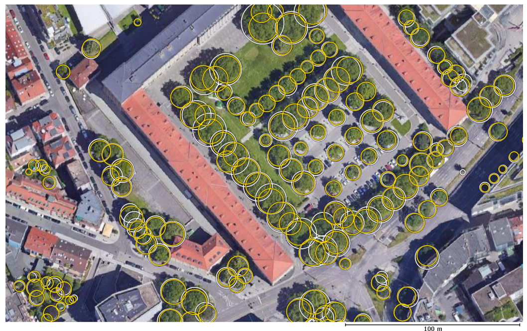
Figure 3. Exemplary detections from SCN-OD-RG in the test set. Yellow: predictions; white: ground truth.
