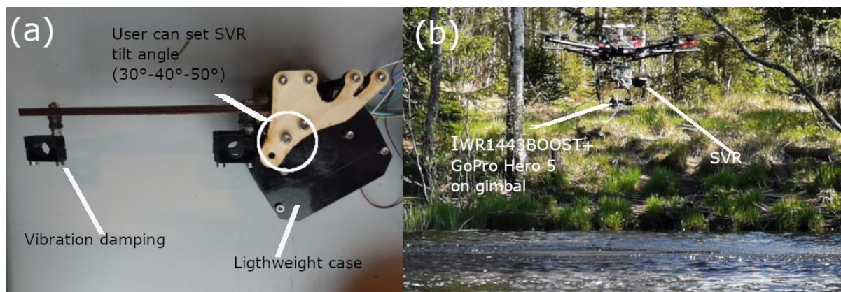
Figure 1. Pictures of UAS payload. (a) SVR adaption for being used as drone payload (b) UAS flight with SVR Doppler radar, IWR1443BOOST radar and GoPro Hero 5 RGB camera.
