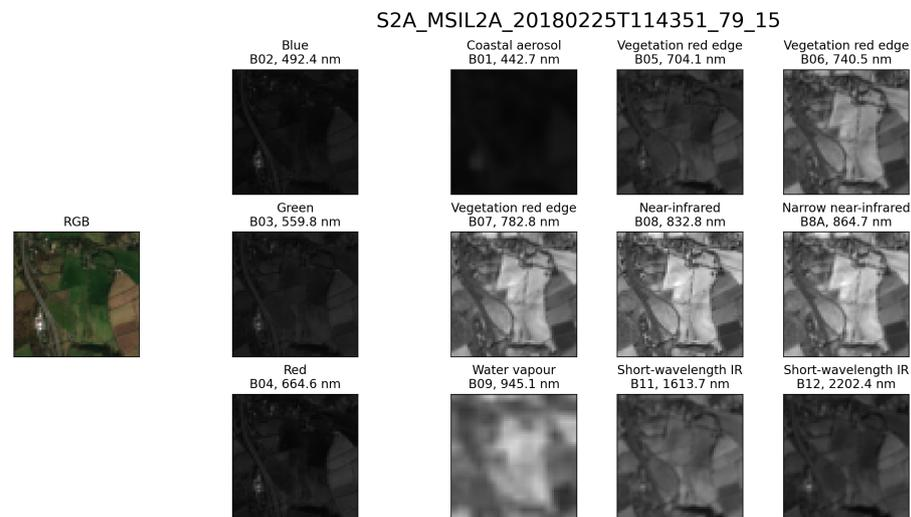
**Figure 1.** Multispectral image captured by the satellite Sentinel-2 and belonging to the BigEarthNet database.
