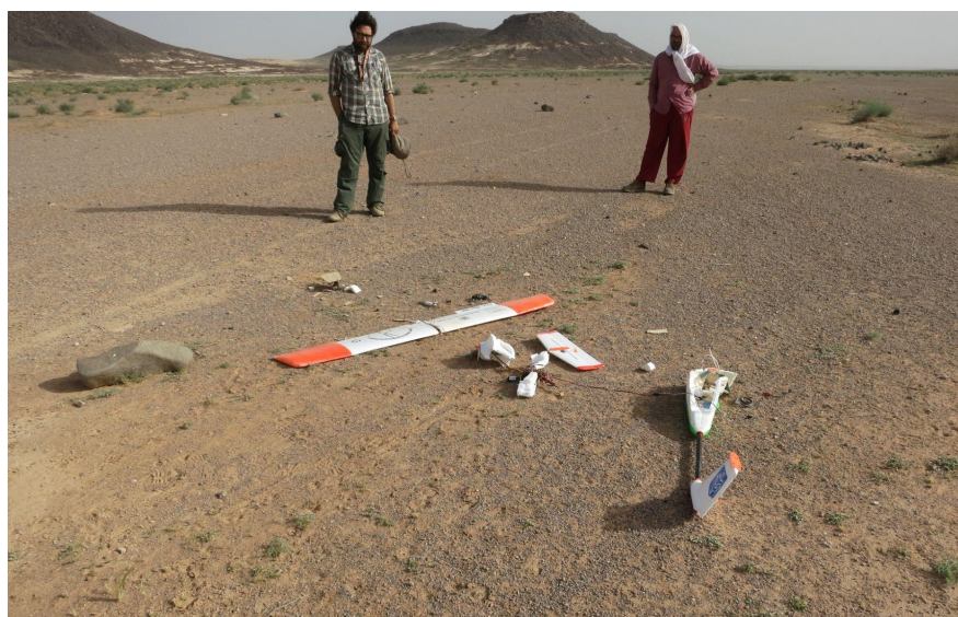
Figure 6. The results of a crash landing of the fixed-wing drone. Repaired by the pilot (Hill), the plane flew again several weeks later.
