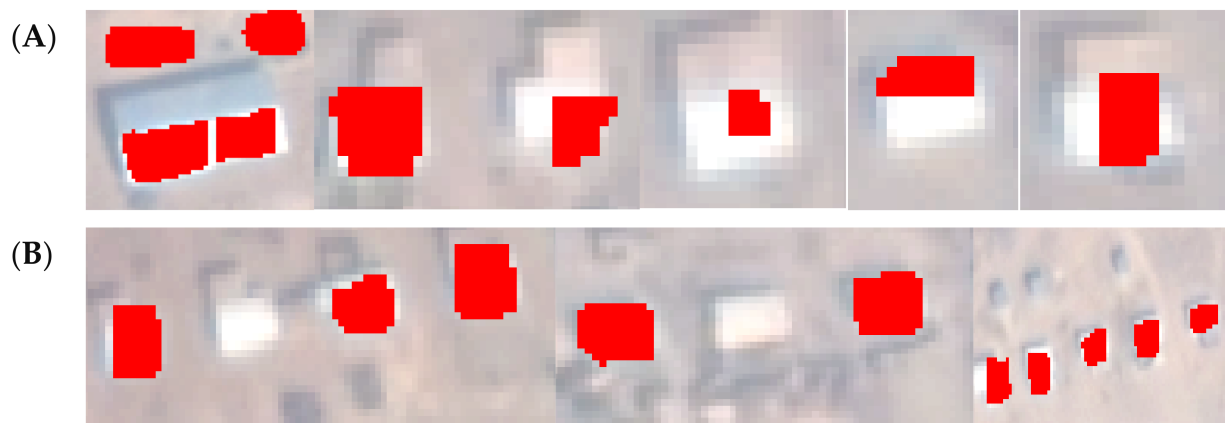
Figure 8. Imperfect predictions of the model: (A) prediction with inaccurate object-boundary localization; and (B) missing dwelling features (false negatives).
