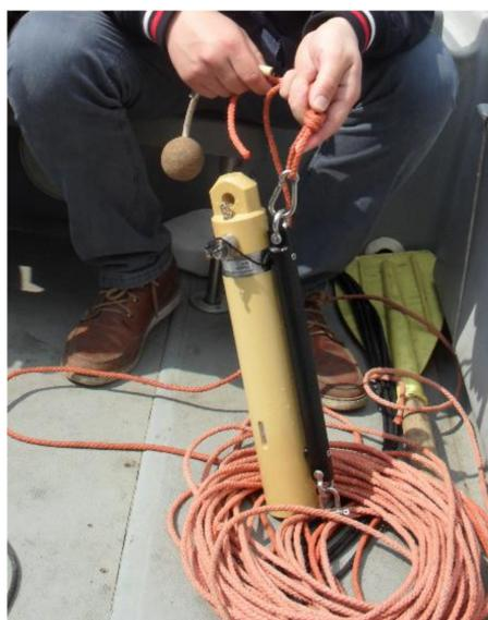
**Figure 3.** STD/CTD probe model SD204.
