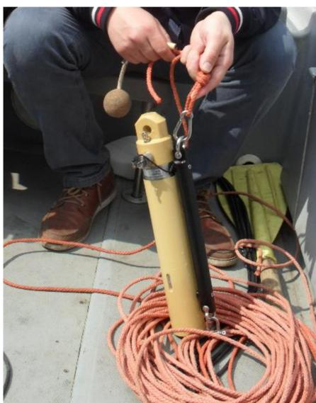
**Figure 3.** STD/CTD probe model SD204.
