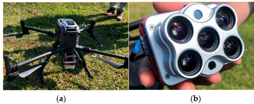
**Figure 3.** (a) DJI Matrice 300 platform, and (b) MicaSense Altum multispectral-thermal camera.
