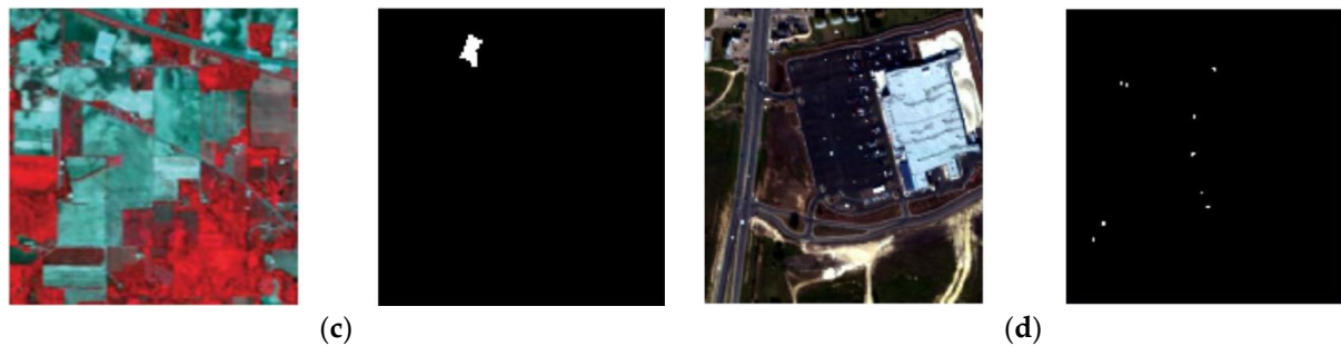
Figure 3. The HSI dataset and the corresponding ground-truth used in the experiments. (a) AVIRIS I dataset, (b) AVIRIS II dataset, (c) The Indian Pines dataset, (d) The HYDICE dataset.
