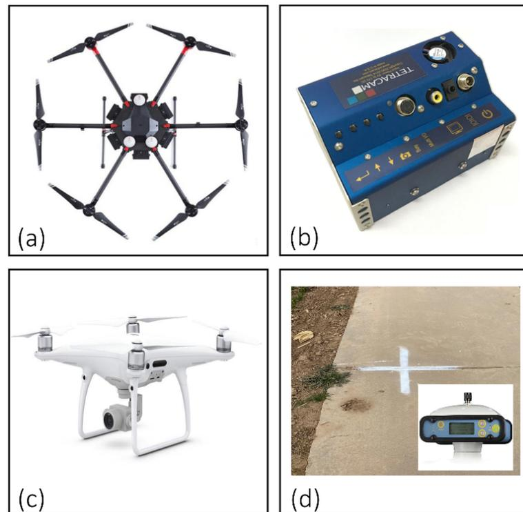
**Figure 2.** The UAV and cameras applied for data collection: (a) DJI M600 Pro UAV; (b) Mini MCA 6 Camera; (c) DJI Phantom 4 Pro V2.0; (d) ground control points.
