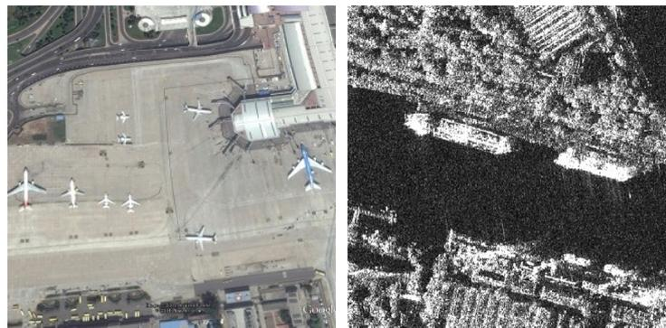
**Figure 5.** Typical remote sensing images. (Left): Optical remote sensing image with airport objects; (Right): SAR image with ship objects.
