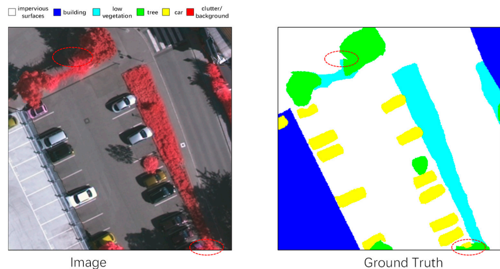
Figure 1. A high-resolution remote sensing sample image and the corresponding ground truth from the ISPRS Vaihingen dataset. The red circle shows the irregularity of the target boundary in the remote sensing images.
