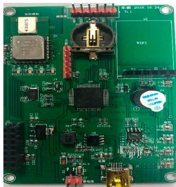
Figure 8. Positioning solution development board.
