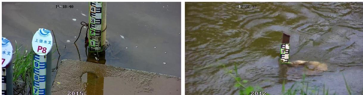
Figure 10. Dirty water gauge image inspection results.
