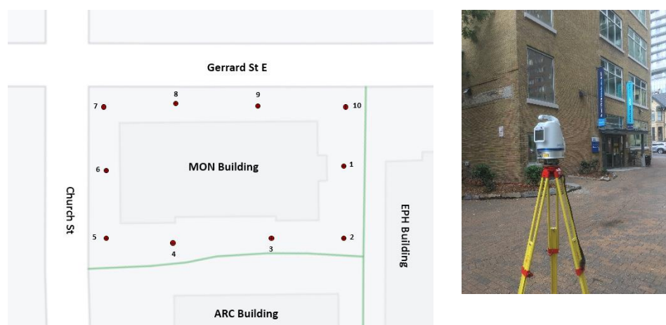
Figure 3. Scans' locations (from 1 to 10) around the MON building (left) and the Polaris system scanning the building from Station #2 (right).
