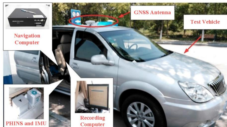
**Figure 2.** Installation diagram for vehicle-mounted experiment.
